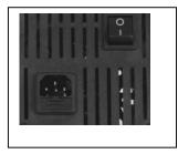
The fuse is located in the pull out drawer underneath the mains inlet socket. A spare fuse can also be found in the drawer. Make sure the mains lead has been removed before opening the drawer.
