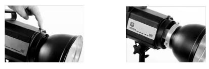
Pull back the spring locking lever as shown and rotate the reflector in an anti-clockwise direction until it is possible to pull the reflector away from the mount. To re-fit the reflector, insert the reflector into the mount ensuring that the hole for the umbrella shaft in the reflector is in line with the corresponding hole in the body. Push the reflector so that the locking lever moves backwards and turn the reflector in a clockwise direction, until it locks into place.
